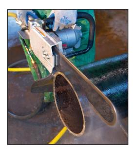
The PowerGrit system allows the user to perform the entire cut from one position – a feature especially helpful in reducing the amount of excavation required in underground cuts.
